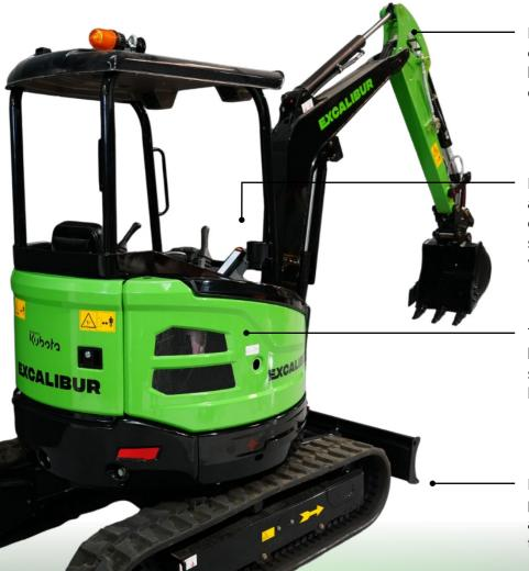
Featuring heavy-duty steel construction and high-flow hydraulics, the stick tackles demanding excavation with ease.
