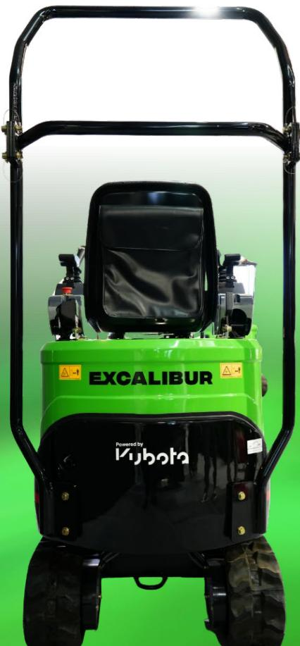
ROPS &amp; TOPS Roll Bar - coupling with ROPS &amp; TOPS specifications.
